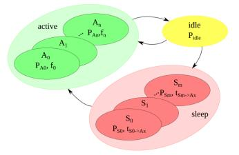
Fig. 1. CPU core state machine
