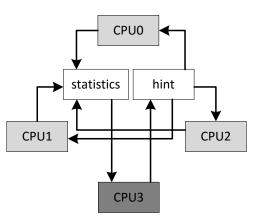
Fig. 7. Architecture of multiprocessor system with 3 worker and 1 manager core, with ability of load balancing
