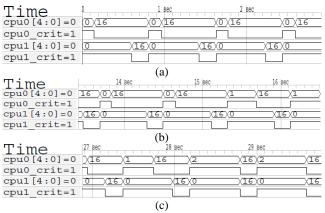
Fig. 9. Load balancing process of different worker cores executing same programming load
